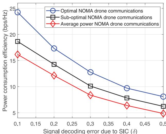
Fig. 4. Impact of signal decoding error on the power consumption efficiency of NOMA drone communications.
