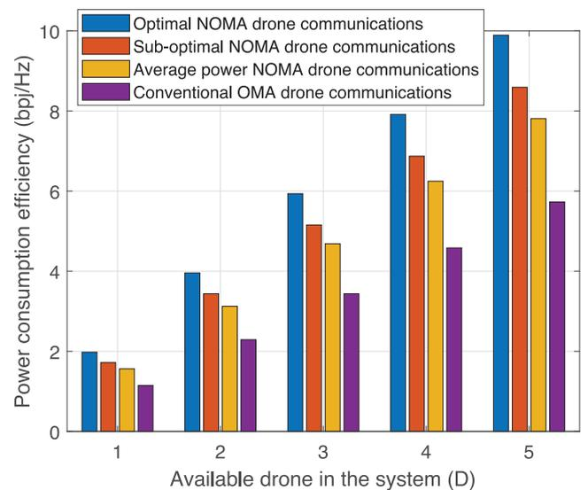
Fig. 3. Increasing number of drones versus power consumption efficiency of the system.
