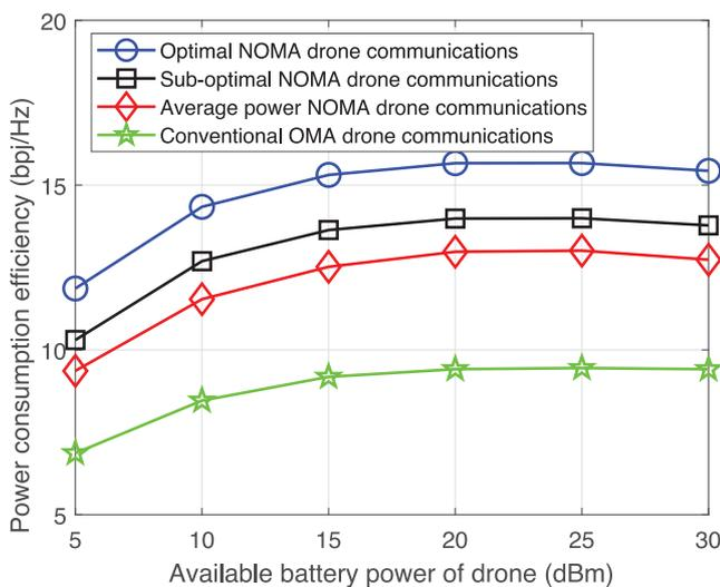
Fig. 2. Impact of available battery power on the power consumption efficiency of drone communications.
