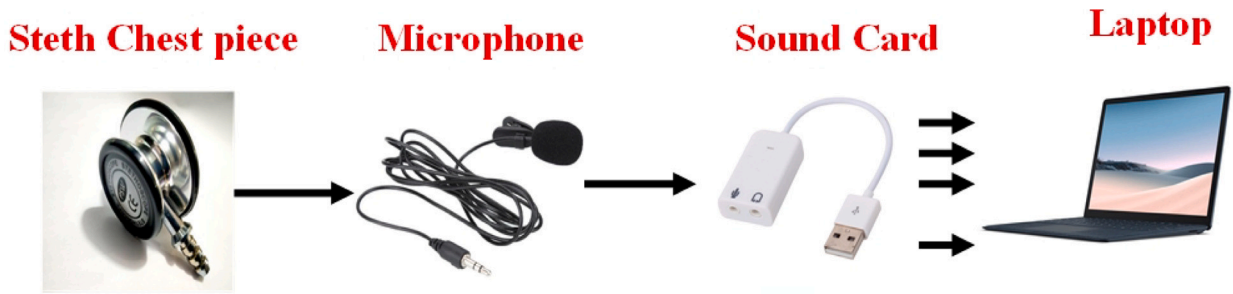
Fig. 1. Block diagram of self-designed PCG Acquisition System (PAS).
