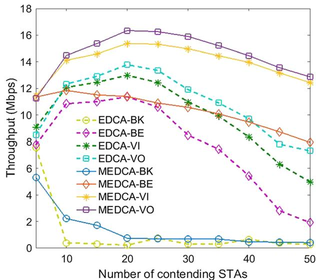
Fig. 7 Throughput comparison of EDCA and MEDCA for different ACs (BK, BE, VI and VO)
