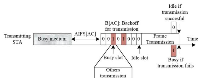
Fig. 2 Channel observation-based collision probability according to COSB [14]
