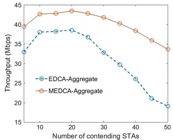
Fig. 8 Aggregate system throughput comparison between EDCA and MEDCA
