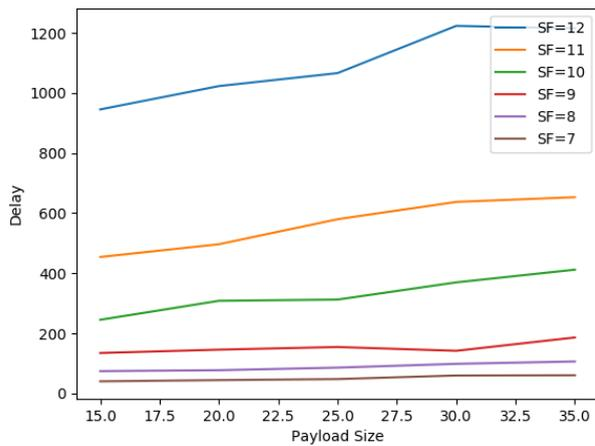
FIGURE 9. Delay w.r.t Payload Size for different SFs.
