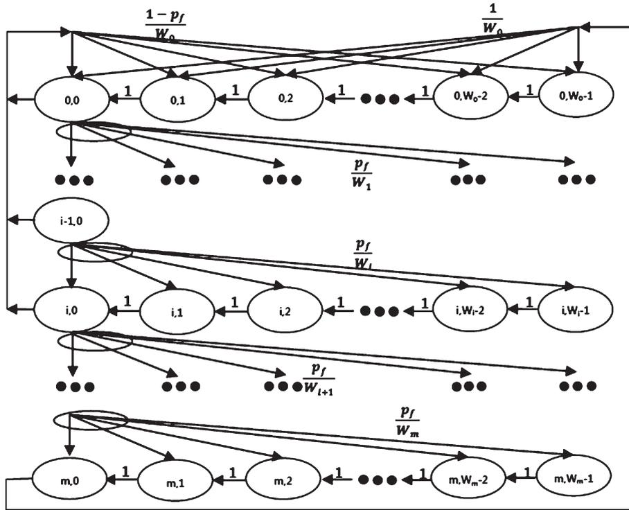
Fig. 4. Markov chain model for the backoff stage in the GCR block ACK scheme.
