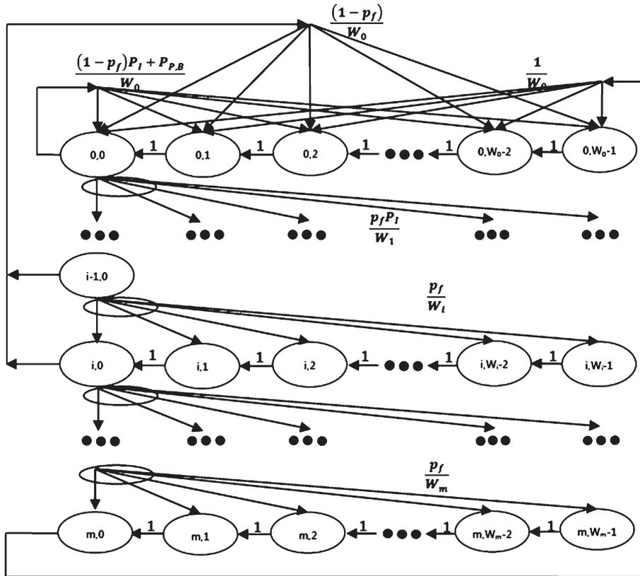
Fig. 5. Markov chain model for the backoff stage in proposed scheme.
