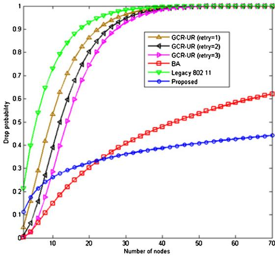
Fig. 8. Average drop probability as a function of the number of nodes.
