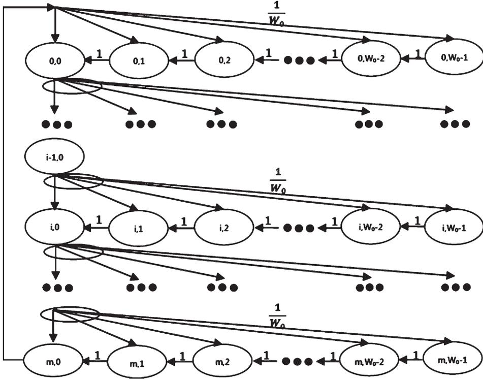
Fig. 3. Markov chain model for the GCR-UR scheme.
