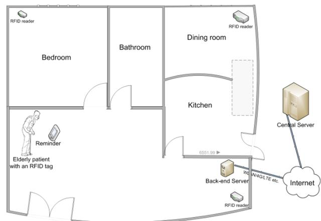
**Figure 1.** General Framework of RFID Deployment in Elderly Home.
