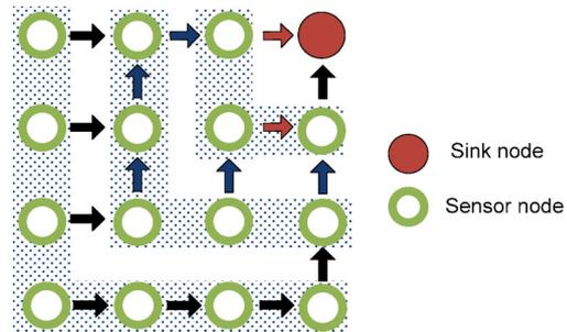
**Figure 11.** The shadow region marks the L-Layer partitions. A tree is constructed for a  $4 \times 4$  grid-based WSNs [15].
