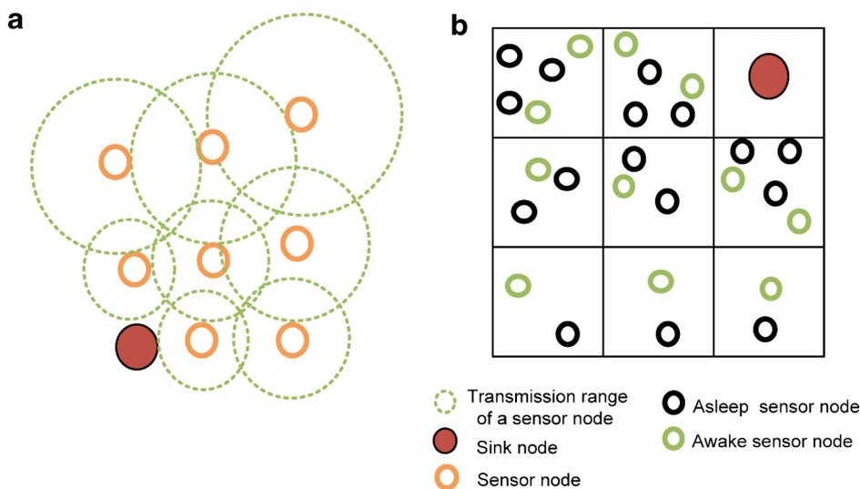
Figure 8. (a) The distance-based mechanism, (b) the density-based mechanism [15].
