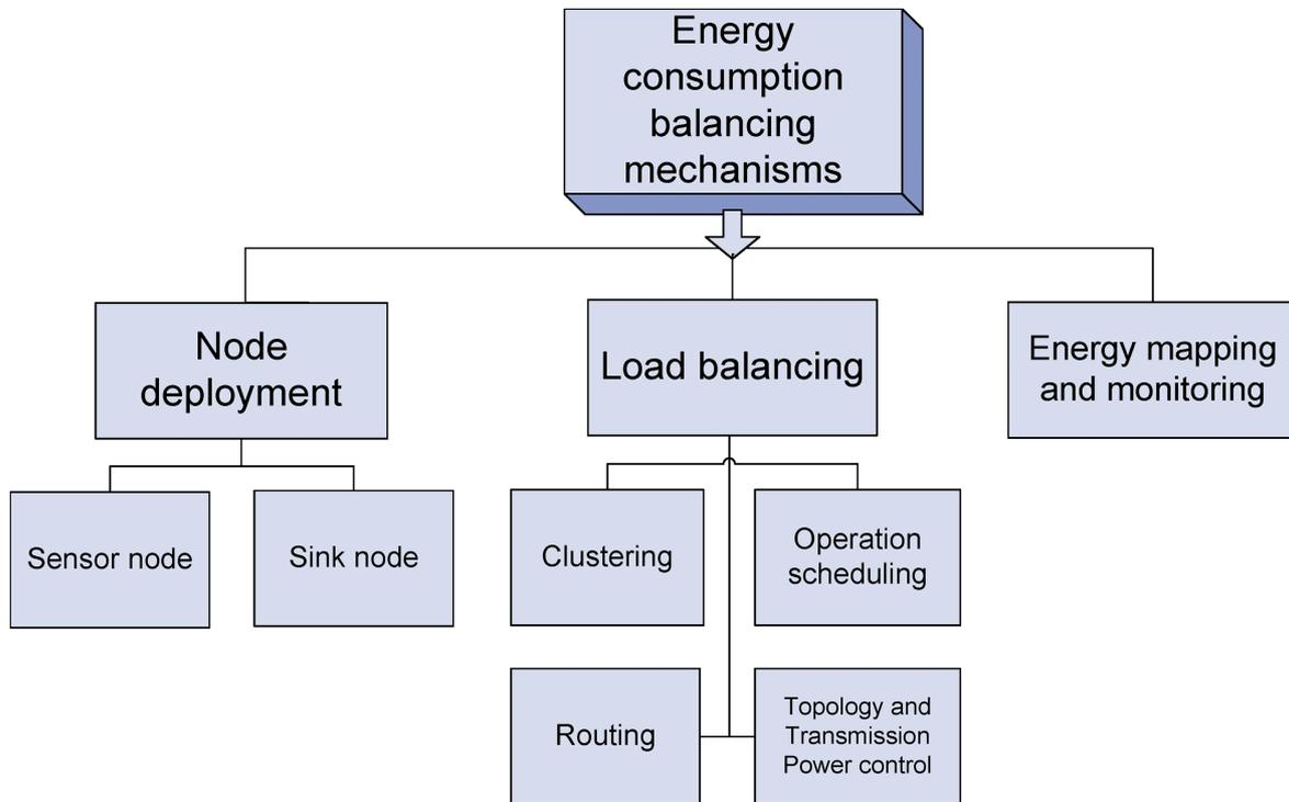
Figure 5. Classification of ECB mechanisms.
