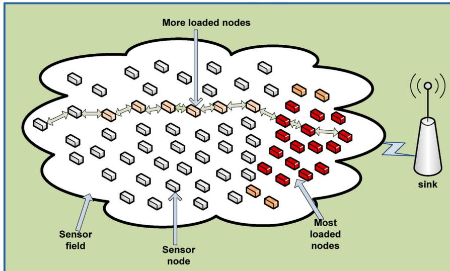
**Figure 1.** Example of unbalanced energy consumption among nodes using multihop mode communication in WSN.
