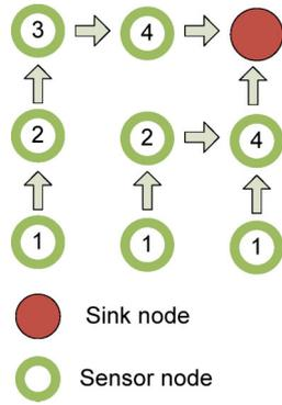
Figure 7. A 3 × 3 grid-based WSN. A root-balanced tree is constructed [15].
