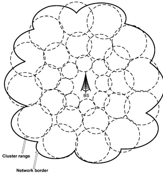
**Figure 9.** Conceptual figure of unequal clustering.
