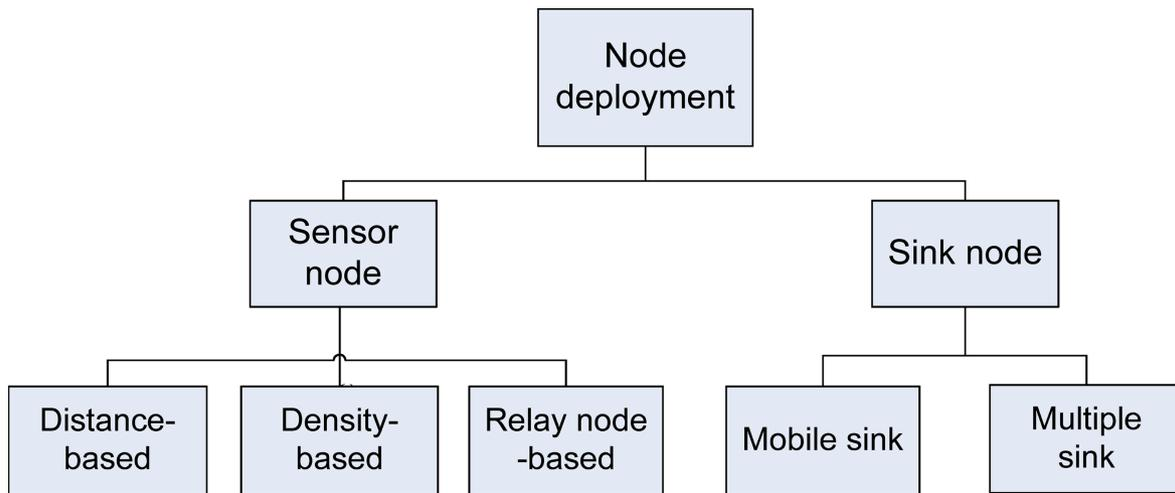
Figure 6. Classification of ECB node deployment mechanisms.
