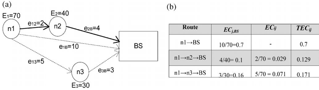
**Figure 10.** Example scenario to demonstrate routing algorithm: (a) node n1 needs to send data to BS; (b) three routes and the route through n2 is best candidate.
