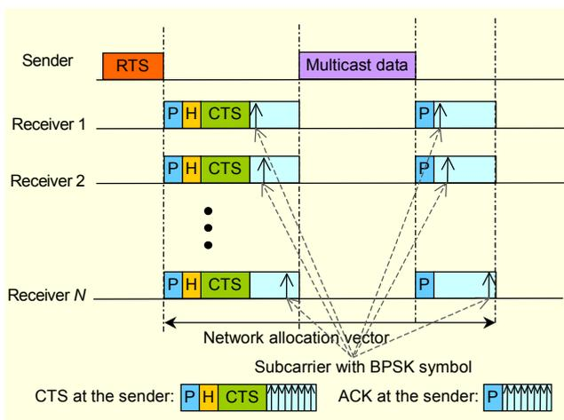
Fig. 2. Example of a data packet transmission cycle.
