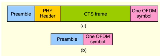
Fig. 1. (a) CTS and (b) ACK packet format.
