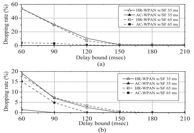
Fig. 7. Effect of the packet delay bound on the packet dropping rate: (a) CBR traffic, (b) VBR traffic.
