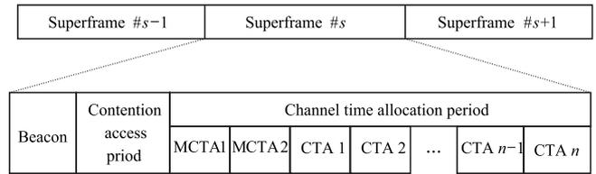
Fig. 1. Superframe structure of IEEE 802.15.3.
