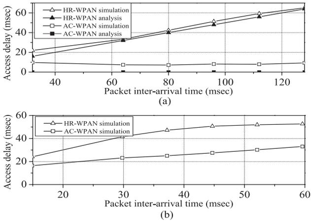
Fig. 5. Effect of the packet inter-arrival time on the mean access delay: (a) CBR traffic, (b) VBR traffic.
