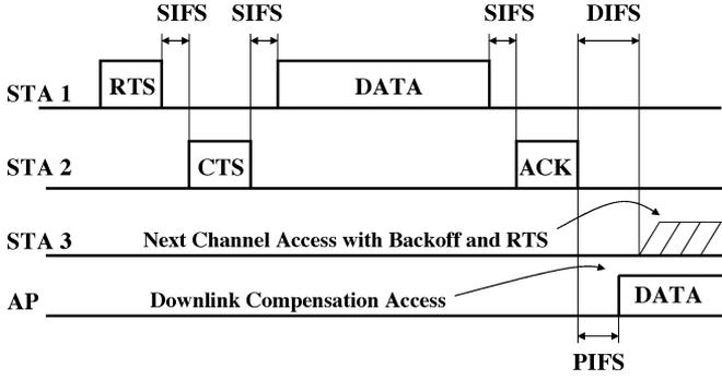
Fig. 1. DCF access mechanism and downlink compensation access mechanism.
