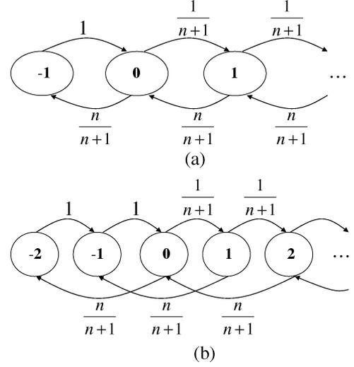
Fig. 3. State transition diagram for  $\omega(t_s)$  at (a)  $\psi = 1$  and (b)  $\psi = 2$ .
