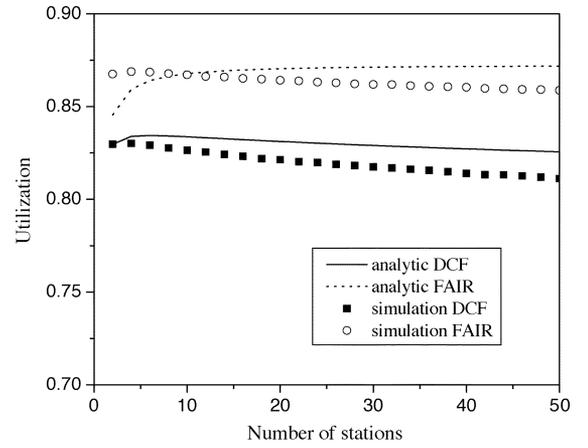
Fig. 5. System utilization  $U$  of analysis and simulation at  $\psi = 1$ .
