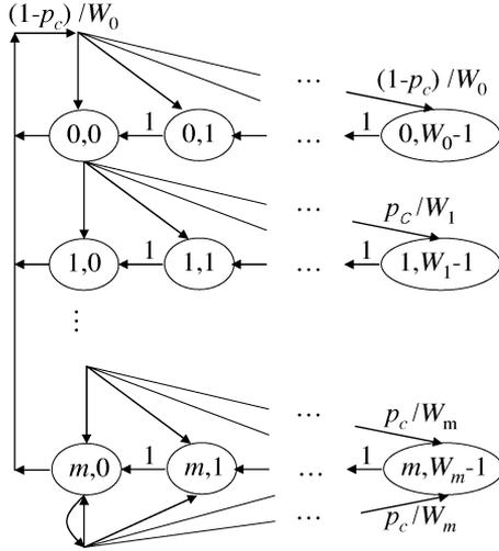
Fig. 2. State-transition diagram for the backoff window size.
