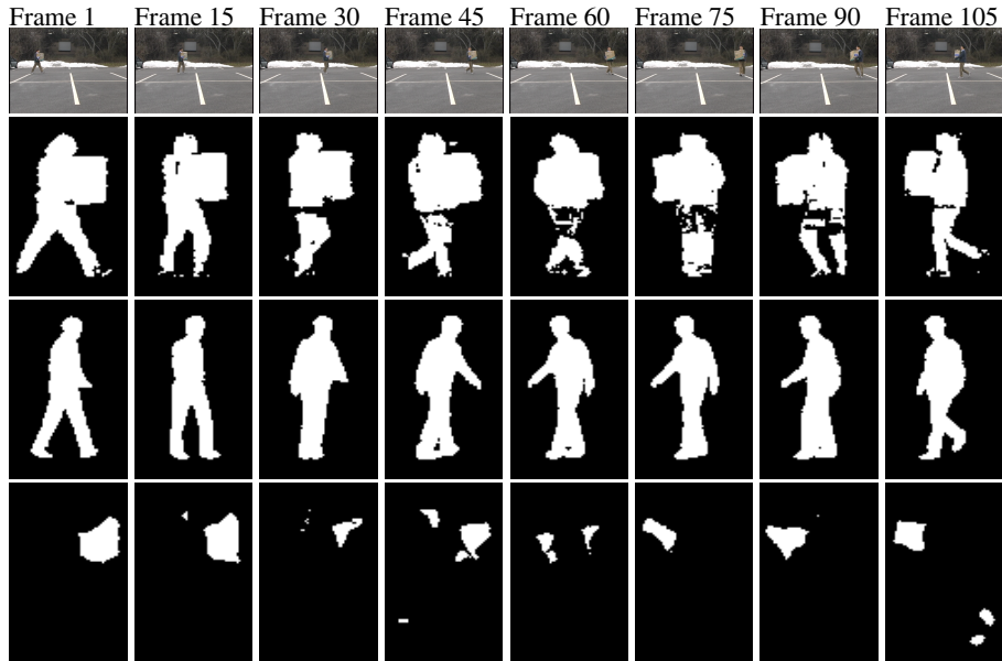
Fig. 4. Outlier detection in continuous view variations: First row: Input image. Second row: Extracted silhouette shape. Third row: Best matching shape. Fourth row: Detected carrying objects.
