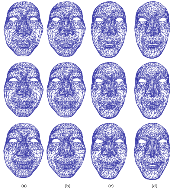
Figure 7: Expression and geometry morphing. Col.(a): Second actor’s original motion sequence, \alpha = 0 . Col.(d): First actor’s original motion sequence, \alpha = 1 . Col.(c): Morphing result with \alpha = 0.2 . Col.(d): Morphing result with \alpha = 0.8 . From top to bottom, rows shows sampling of the generated motions at the 1st, 25th and 50th frame out of the 150 total frames.
